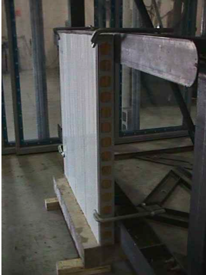
RBS4 Test Panel Clamped to Reaction Frame
